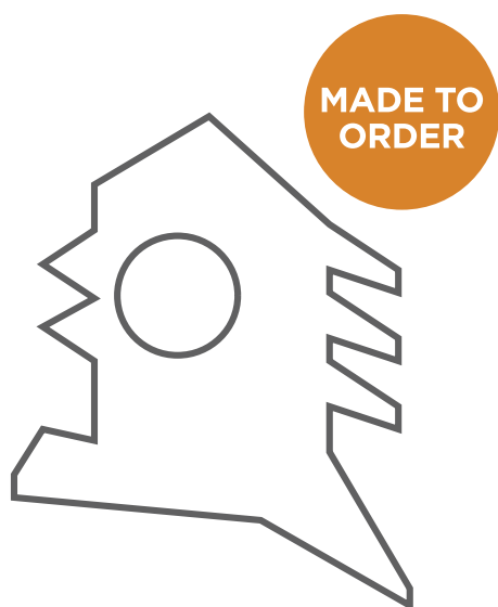
Drawing Number D0776 Part Number 01500776 Material EPDM
