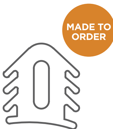
Drawing Number D03660 Part Number 01500001E068 Material EPDM
