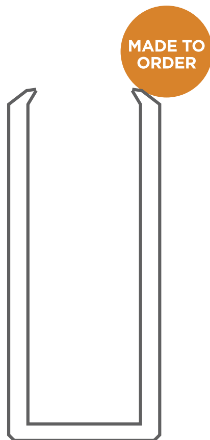
Drawing Number D03662 Part Number 01100038E038 Material EPDM
